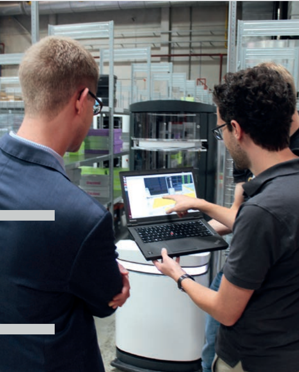
The robot transports the shoe box autonomously from the rack to the person.
